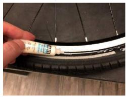
Step 1: Pour the bead butter between the rim and the tire.
