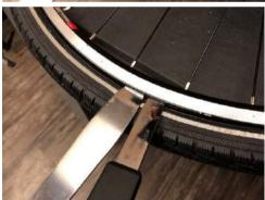
Step 3: Insert the tire lever, will feel "click" when lock on the bead.
